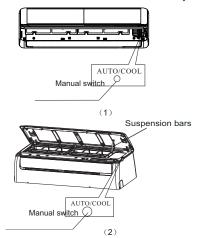
**NOTE:** The unit must be turned off before operating the manual control button. If the unit is operational, continue pressing the manual control button until the unit is off.
