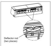
Adjust the air flow direction properly otherwise it might cause discomfort or cause uneven room temperatures.
